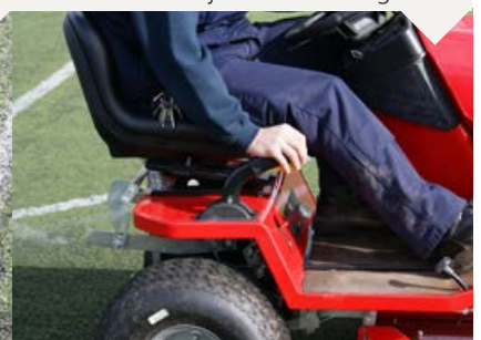
Brush can be lifted and pressure adjusted from a single lever
