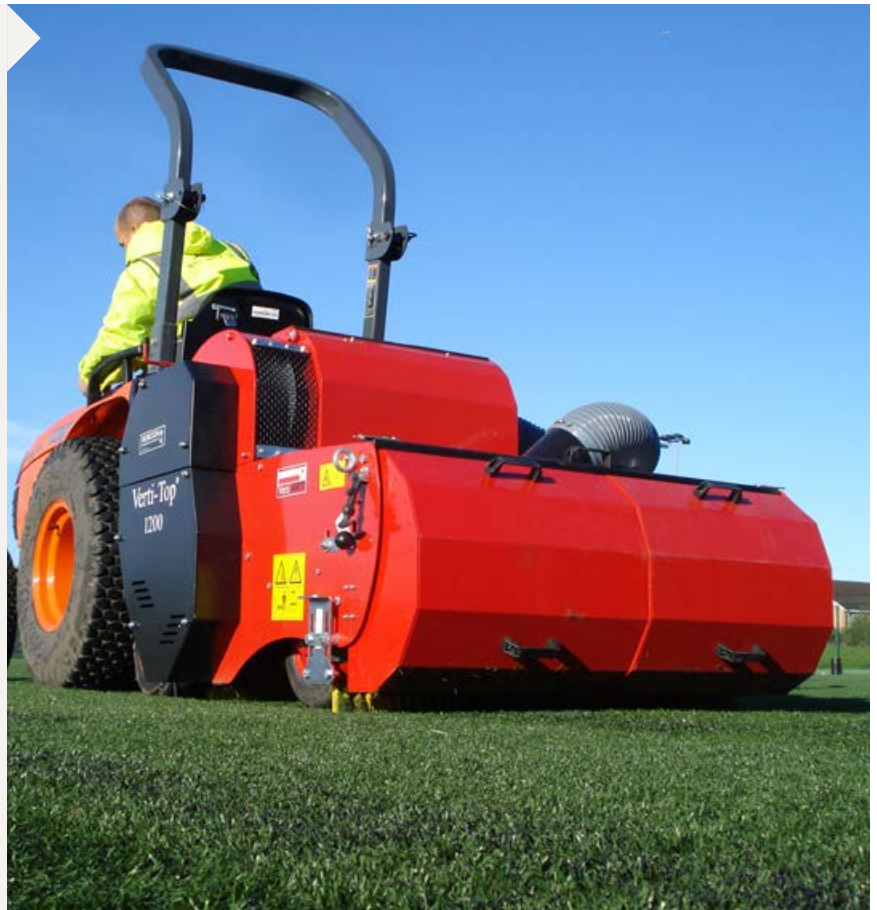
Intensive action lifts infill and restores playing characteristics
