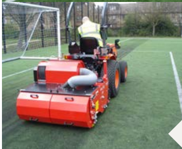
Intensive action lifts infill and restores playing characteristics
