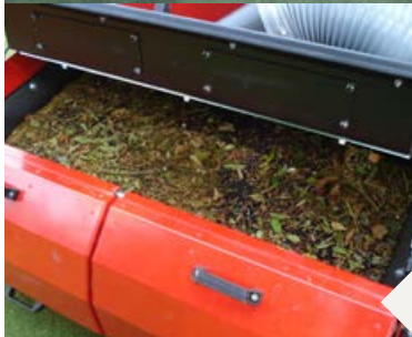
Sieve separates infill from debris and detritus
