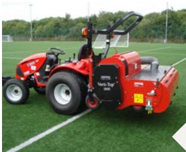
Verti-Top can be operated from a 20hp tractor
