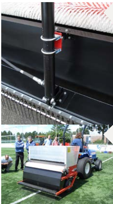
Hydraulic ram, lifts and lowers the grooming rakes
