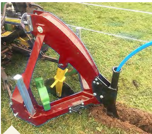
The Mole-Plough can easily be mounted with a pipe laying Leg.
