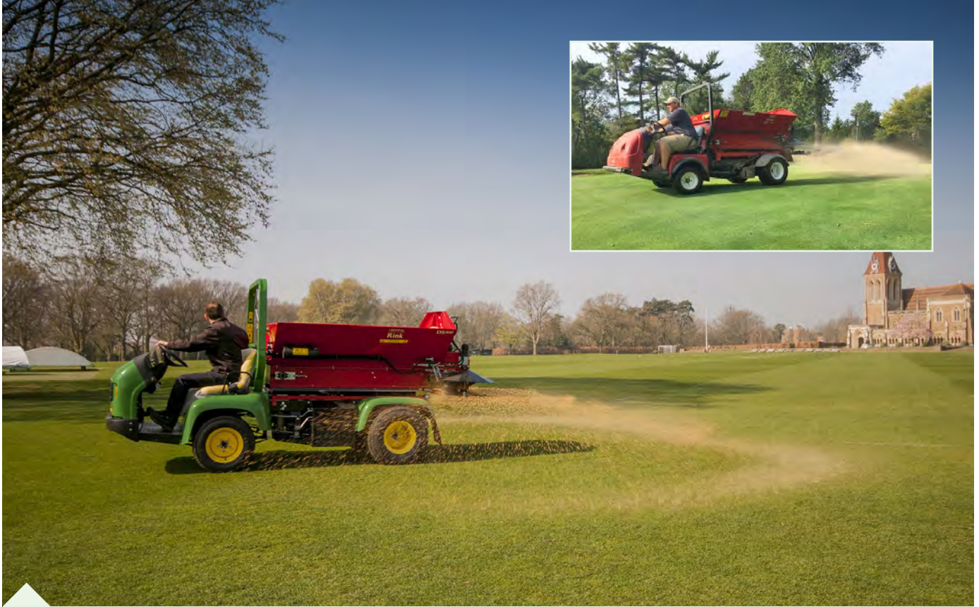
The Rink DS800 can be mounted to either a Toro Workman or John Deere Progator.
