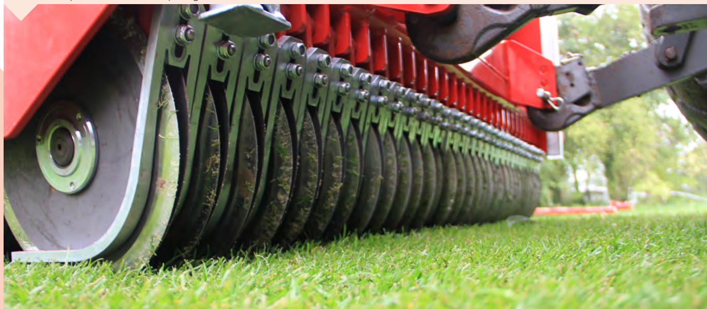
Double discs provide a 3cm seed spacing.
