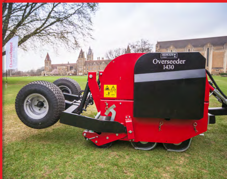
Double discs provide a 3cm seed spacing.
