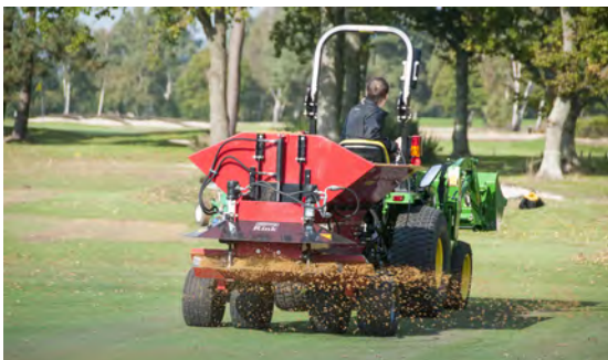
DS800 trailed, this disc spreader has a hopper capacity of 0.8m 3 . The operation of the belt and spinners is carried out from the tractor seat.
