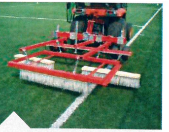
Floating brush unit allows the bristles to re-erect fibre
