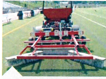
The brushes lift and level infill behind the Verti-Groom unit
