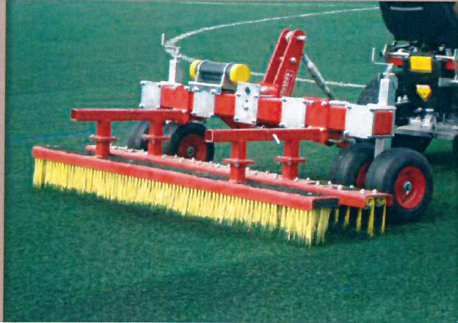
The brushes lift and level infill behind the Verti-Groom unit
