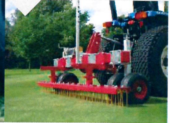
5mm tines are suitable for more aggressive de-compaction and use on natural turf surfaces
