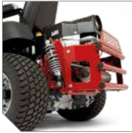
Rear suspension with coil-over-shocks and pivoting front axle with motion dampening shocks.
