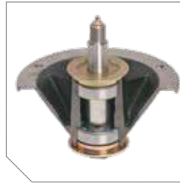
Cast-Iron Spindles longer usable life, 25,4 mm shaft with top access grease fitting for greaseable dual ball bearings, six-bolt 203 mm flange design adds strength and greater dispersal of energy to deck assembly.
