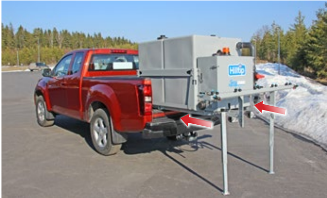
Optional legstand and sliding-tracks on truck bed for easy installation and removing of sprayer.
