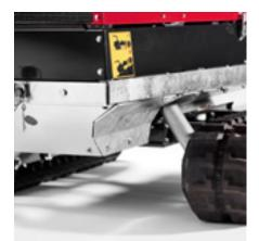
Best Ground clearance on market: 200mm Track width: 1150-1300mm. Reinforced hose protection.
