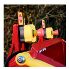
TP E-STOP is standard for operator safety
