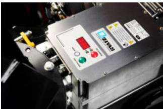
Integrated charger: 230V 16A 65V and cable City and Eco-friendly LMC engine. Reduced noise level.
