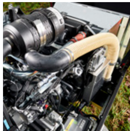
Hatz 4H50 Stage V engine with 55.0 kw
