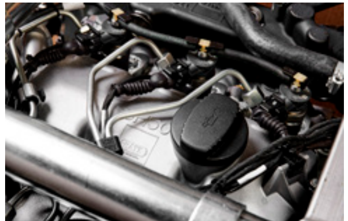
Hatz engine from Germany, Stage V with Bosch common rail system
