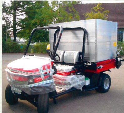
A Hopper Extension Kit can be mounted on top of the Rink 1204, increasing its total capacity to 2.0m 3 for infill (photo left).
