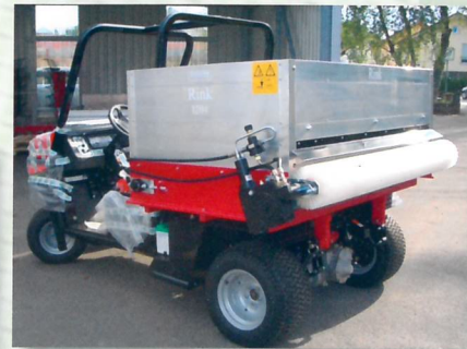
A Hopper Extension Kit can be mounted on top of the Rink 1204, increasing its total capacity to 2.0m 3 for infill (photo left).
