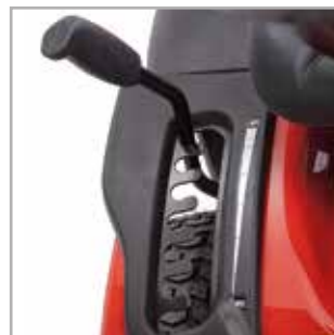
HEIGHT-OF-CUT The manual height-of-cut allows for easy adjustment between 7 possible positions ranging from 4.5 to 9.0 cm.
