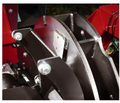
TP OPTICUT<sup>™</sup>: The divided blade system ensures that there is always a blade engaging the wood. The result is less vibration, a more steady strain on the machine, lower fuel consumption level and a more uniform wood chip quality.
