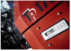
TP PILOT<sup>™</sup>: The main purpose of the stress control system is to prevent the tractor from overloading. Likewise, the system enables monitoring of the speed of rotor disc and feed rollers. The system also includes an hour meter.
