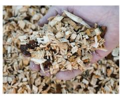
The end product is a first class quality wood chip from 4 to 10 mm. The chip size is hydraulically adjustable.
