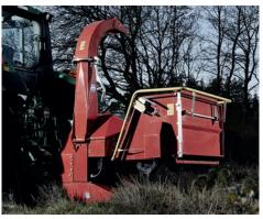
TP 200 PTO is equipped with a folding funnel with the operating bar hinged at the top. The ejector spout is rotatable (300 degrees).
