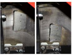
The 4 TP OPTICUT<sup>™</sup> blades are placed alternately on the inner and outer part of the disc. This way, a blade is always engaging the wood, causing fewer vibrations, lower fuel consumption and a uniform wood chip.
