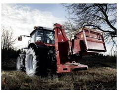
TP 250 PTO is equipped with a folding funnel with the operating bar hinged at the top. The ejector spout is rotatable (300 degrees).
