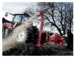
The end product is a first class quality wood chip from 4 to 13 mm. The chip size is hydraulically adjustable.
