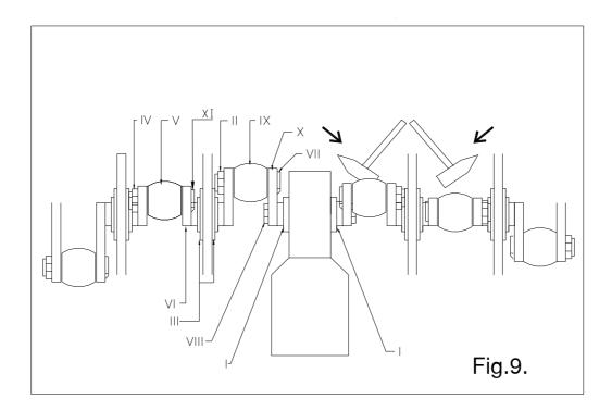
In fig.9. the assembly of the crankshaft is given. Also look at the spare part page for a more clear view and setup. On a 7212 the angle between the handles on the gearbox should be 67.5 degrees.
