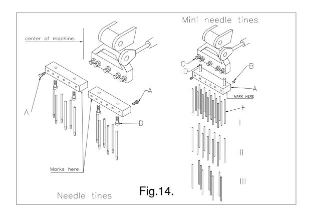
Mini Needle (solid) tines need a mini needle adapter block. The two studs D ( fig 14, right) fit a  $12 \text{ mm} (\frac{1}{2})$  hole C of the standard machine tine head.
