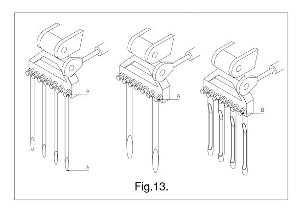
Shorter (worn) tines can be used in case shallower penetration is required. The machine doesn't need to be adjusted that much at that time. Note that the depth reading on the decal is only correct when using the full maximum length tine
