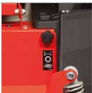
STEERING LEVER TRACKING ADJUSTMENT Adjusting the steering levers so that your zero turn tracks straight.
